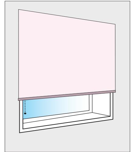
**FACE FIT** is where the blind will be mounted on the wall or window frame and will cover the total window area.
